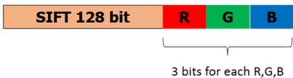
Fig. 6 Moment color-SIFT descriptor with 9-bit RGB format
