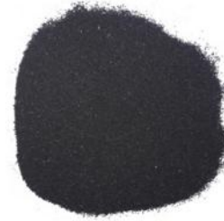
Fig. 2 Crumb rubber used in this research
