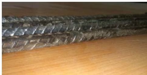
Fig. 4 Cleaned rebars after corrosion
