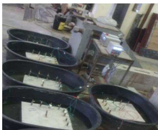
Fig. 1 Accelerated corrosion apparatus for slab elements
