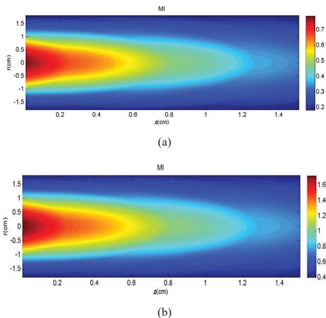
Fig. 2 Ultrasound MI contour of 40 kHz in the r-z, intensity of (a) 0.28 W/cm<sup>2</sup>, (b) 1.34 W/cm<sup>2</sup>: The vertical axis (r) and the horizontal axis (z) show the radial and axial lengths in cm; Color map from blue to red indicates increase in MI
