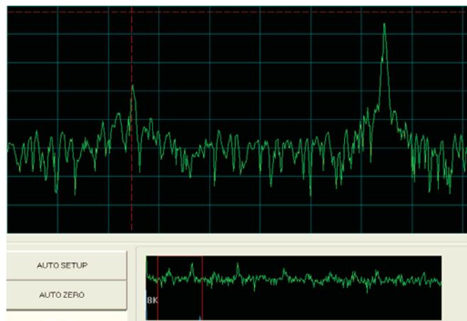
Fig. 1 A sample of the spectrum of 40 kHz with an intensity of 1.34 W/cm<sup>2</sup> in 0.5 cm distance recorded by Spectrum Analyzers; the horizontal axis shows frequency (Hz) and the vertical axis is acoustics pressure (MPa)
