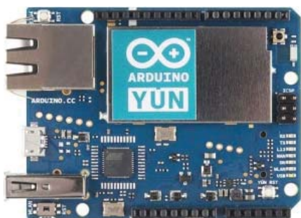
Fig. 4 Arduino Yun used in the experiment as the main processor
