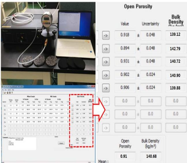
Fig. 5 The measurement of bulk density
