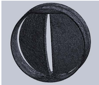
Fig. 3 Mesh from CT scanner
