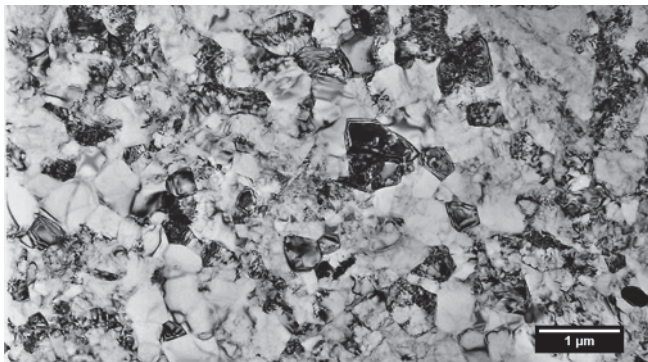
Fig. 5 The structure of Ti Grade 2 upon three passes through CONFORM SPD; the mean grain size is 390 \pm 150 nm
