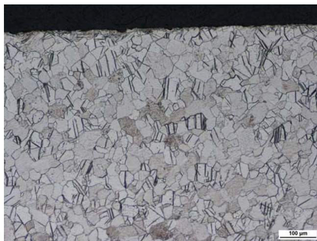
Fig. 3 The initial structure of Ti Grade 2 with the mean grain size of 62 μm
