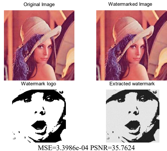
Fig. 10 Example of Image (Lena) watermarking using the proposed technique
