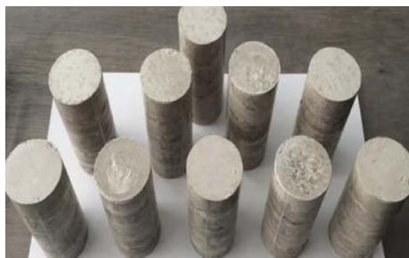
Fig. 3 prepared specimens for UCS test
