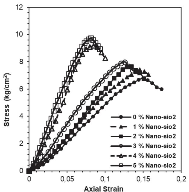
Fig. 4 Stress-strain curves of modified Kaolinite with Nano-SiO<sub>2</sub>
