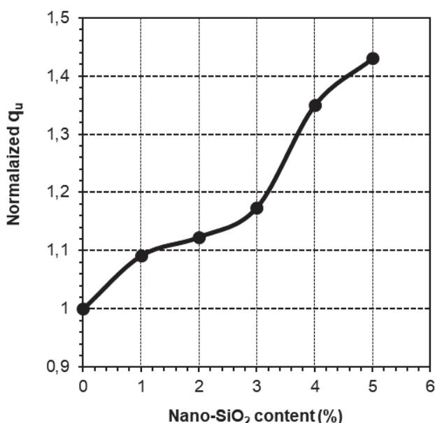
Fig. 6 Variation of Normalized  $q_u$  versus the Nano-SiO<sub>2</sub> content
