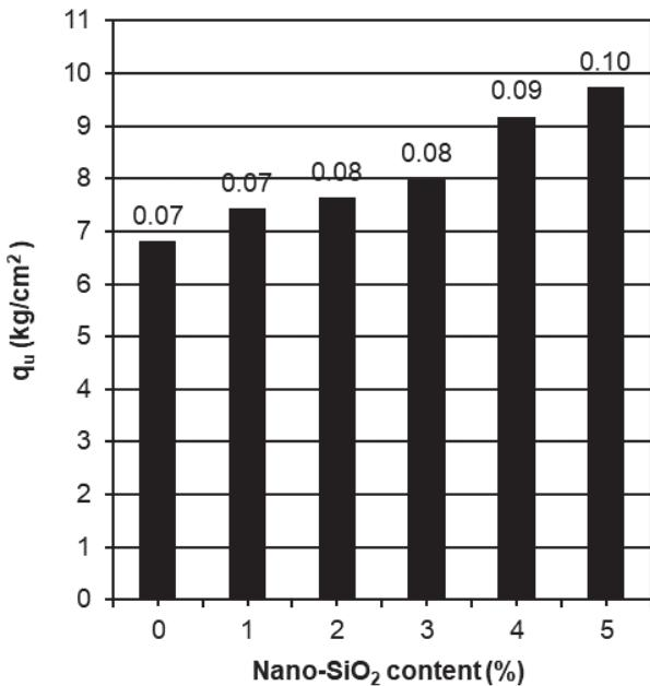
Fig. 5 The effects of Nano-SiO<sub>2</sub> on the UCS of modified Kaolinite
