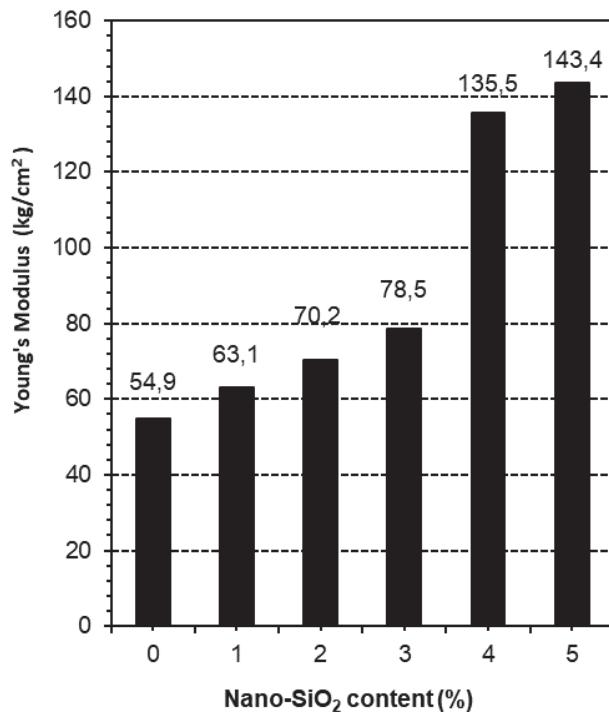
Fig. 7 The effects of Nano-SiO<sub>2</sub> on the Young's modulus of modified Kaolinite
