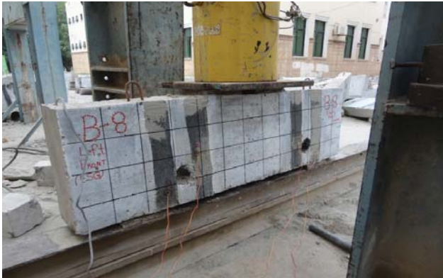
Fig. 5 Loading arrangement for beam testing
