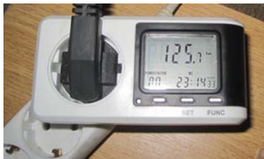
Fig. 6 Monitoring the energy consumption by using the electronic power meter
