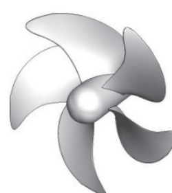
Fig. 1 Geometry of the Seiun Maru HSP propeller
