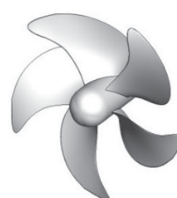
Fig. 1 Geometry of the Seiun Maru HSP propeller
