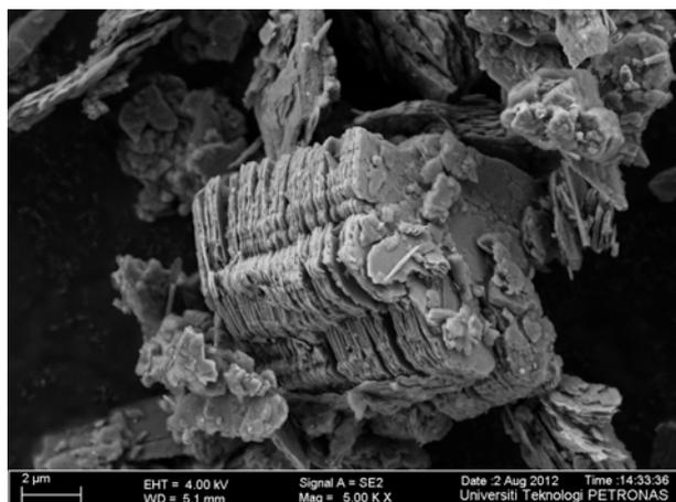
Fig. 2 Microstructure of raw kaolin through FESEM
