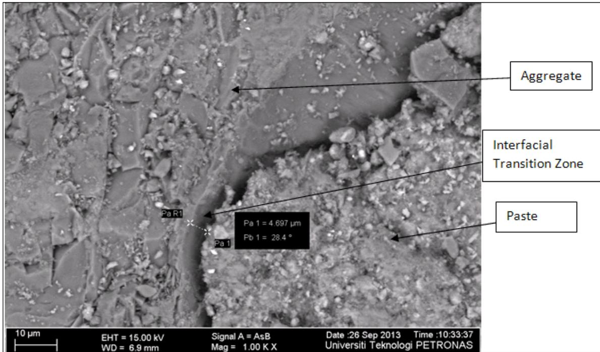
Fig. 5 Microstructure of concrete C-0 through FESEM
