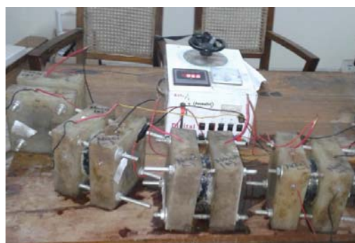
Fig. 2 RCPT test setup
