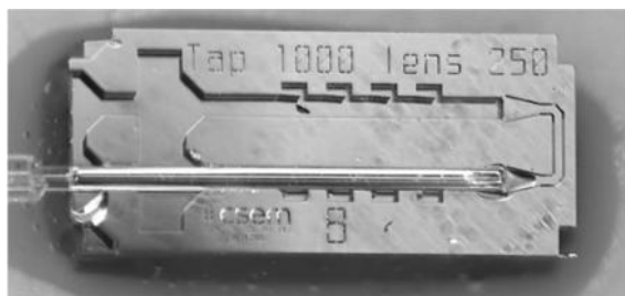
Fig. 7 Assembly of an input fibre with the temperature Si chip
