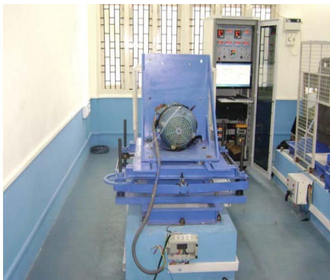
Fig. 9 View of the Motor Test Bed – 2 with 10 HP Motor
