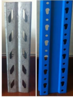
Fig. 1 Arrays of perforations of columns
