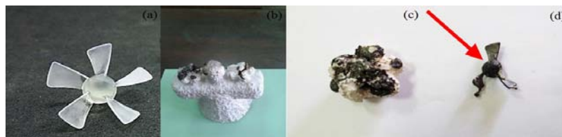
Fig. 7 (a)-(d) Printed ABS resin component, completed shell casting, and product of casting at a temperature of 1700 °C
