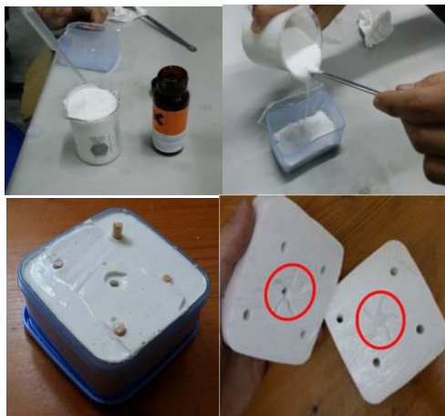
Fig. 5 Creation of silicone mold for wax injection
