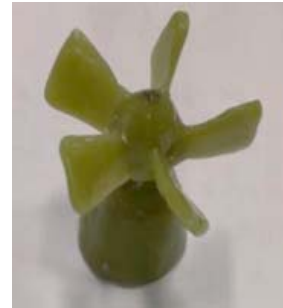
Fig. 6 Product of wax injection
