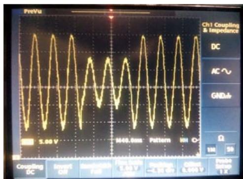
Fig. 11 Voltage sag generated from Disturbances generator
