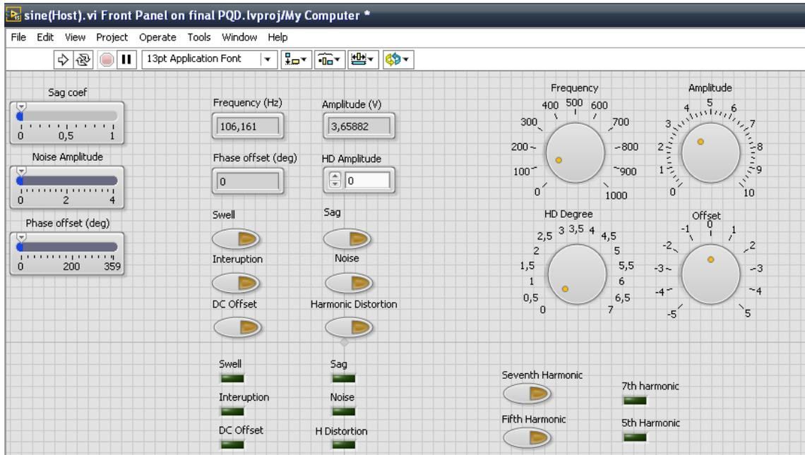
Fig. 3 Host VI Front Panel of Tester
