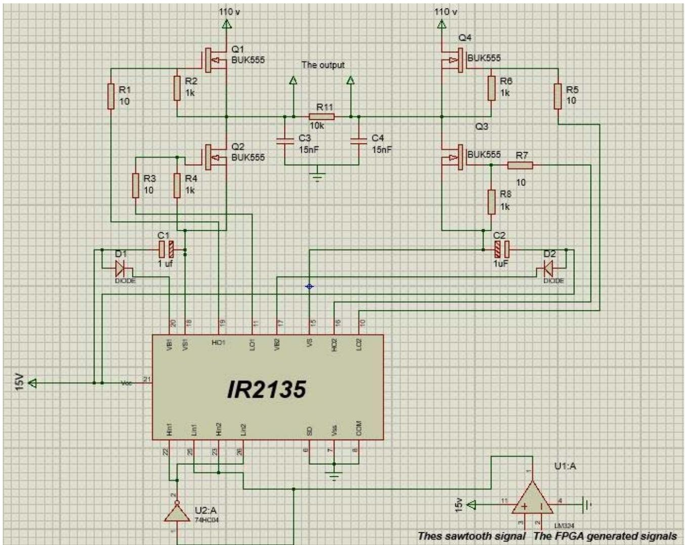
Fig. 6 Class D Amplifier circuit
