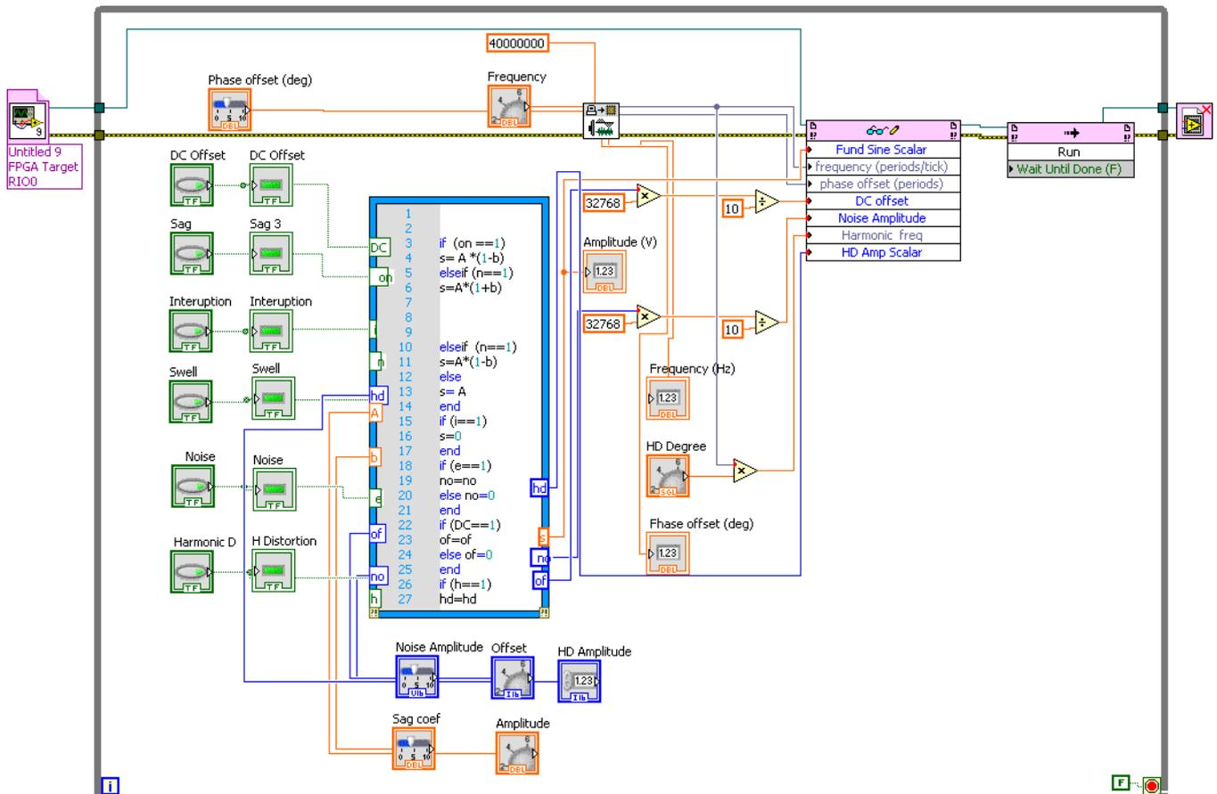
Fig. 4 Host VI Block Diagram of tester.
