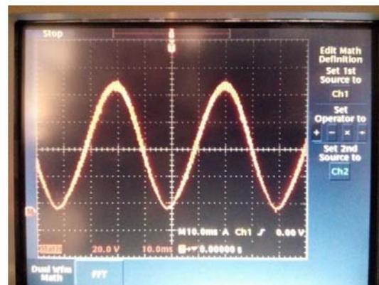
Fig. 9 Output signal of class D amplifier
