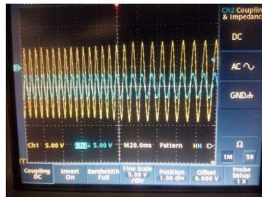
Fig. 10 Amplified sine wave using Class D amplifier
