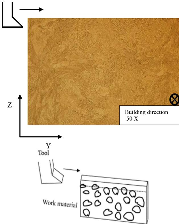
Fig. 4 Microstructural features and the orthogonal cutting strategy employed in machining the case 2 SLM Ti-6Al-4V sample
