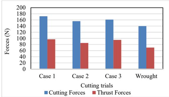
Fig. 6 Forces measured during orthogonal cutting trials
