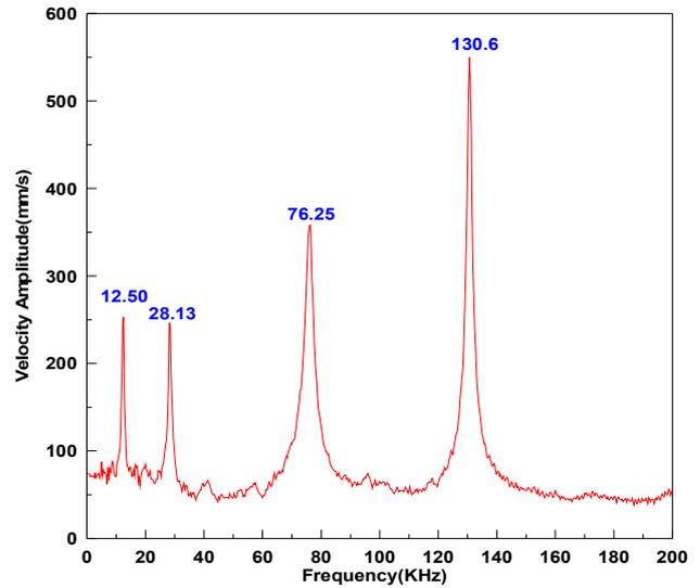
Fig. 3 Frequency response of the vibrating piezoelectric transducer
