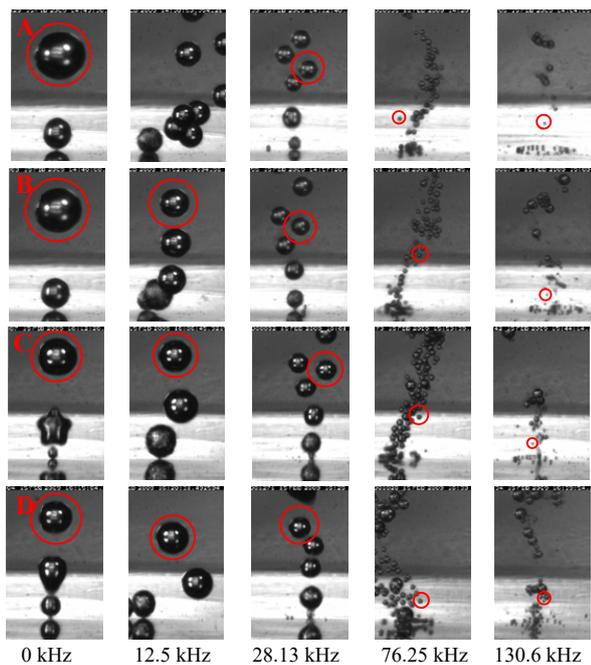
Fig. 7 Sizes of micro-bubble with different driving resonance frequencies. The inlet gas pressure (A) 16.5 kPa, (B) 19.5 kPa, (C) 22.5 kPa, (D) 25.5 kPa. The sinusoidal driving voltage was 80 Vpp
