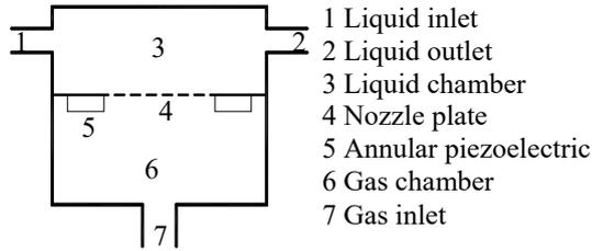
Fig. 1 Illustration of the micro bubble oxygenator
