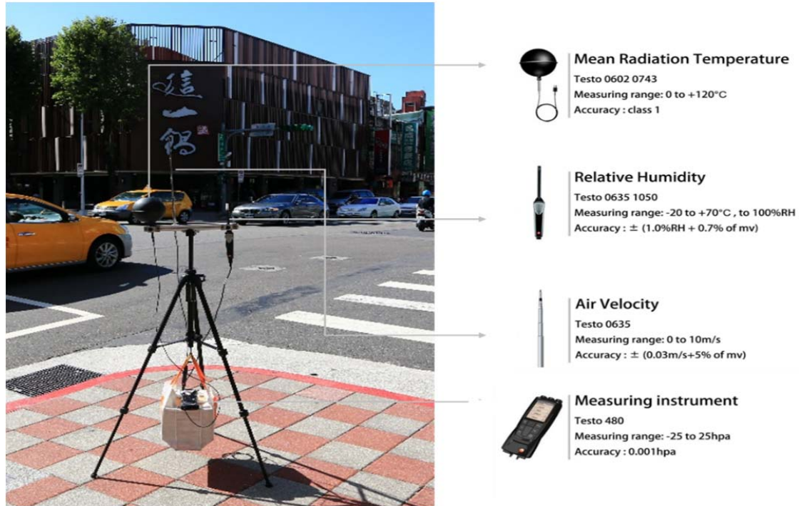
Fig. 2 Measuring instruments and precision introduction
