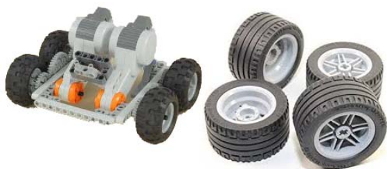
Fig. 2 Mindstorms NXT wheel-mounted motors
