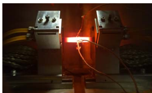
Fig. 2 Sample with thermocouples during heating
