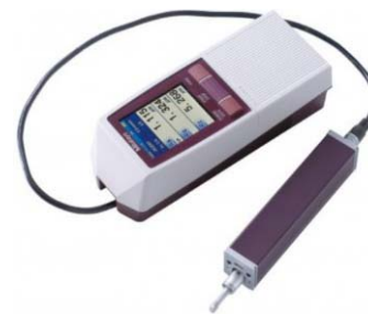
Fig. 3 Roughness meter used to measure surface roughness
