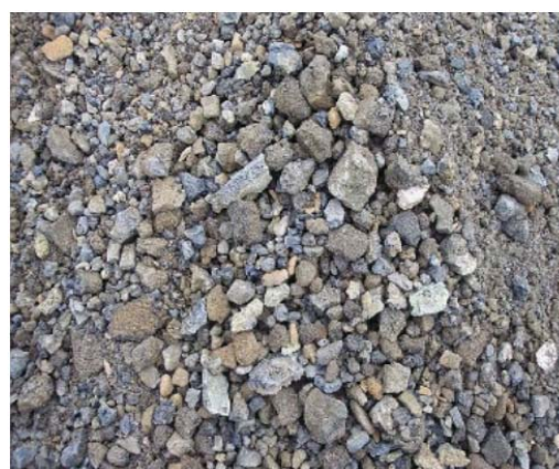
Fig. 1 Bottom ash generated from a thermal power plant
