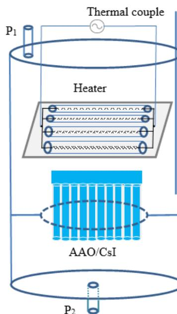
Fig. 2 Schematic diagram of vacuum inhalation chamber
