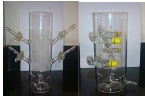
Fig. 6 The beakers used in reactant injection
