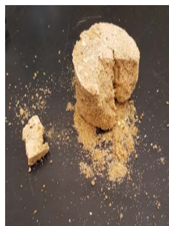
Fig. 8 Sample with high collapsibility potential after treatment from second trail
