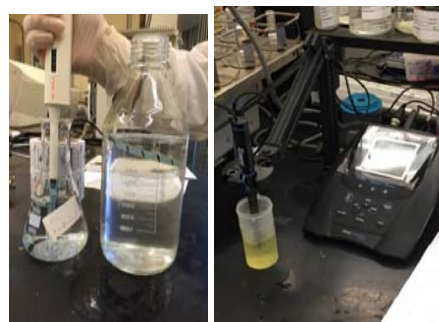
Fig. 2 Adjusting the pH of the Tris buffer
