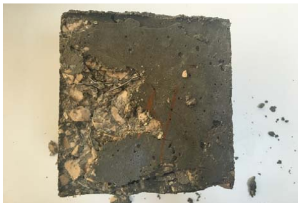
Fig. 3 Cube specimen after compressive strength test
