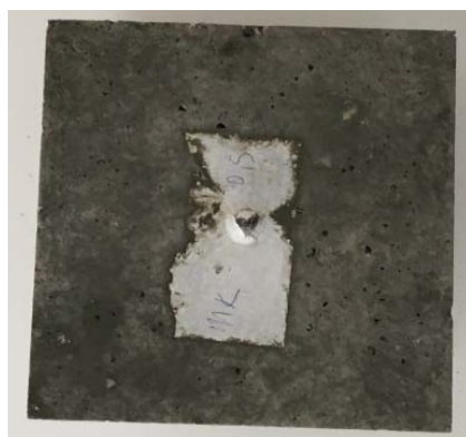
Fig. 5 Cube specimens before compressive strength test
