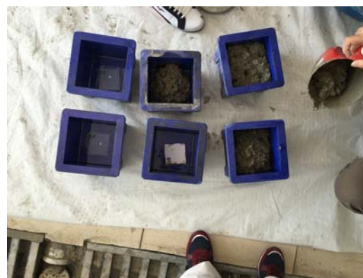
Fig. 6 Preparations of molds before installation
