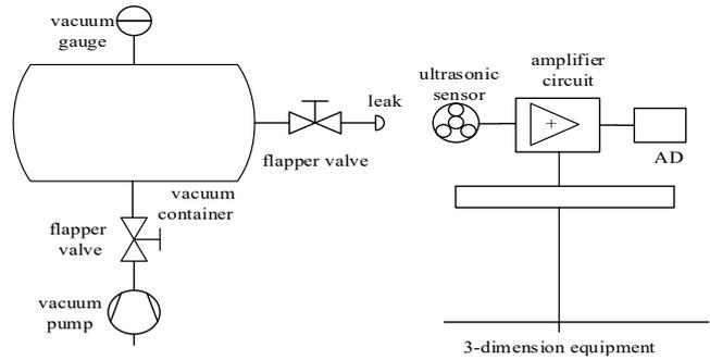
Fig. 4 Diagram of test system for ultrasonic leak detection
