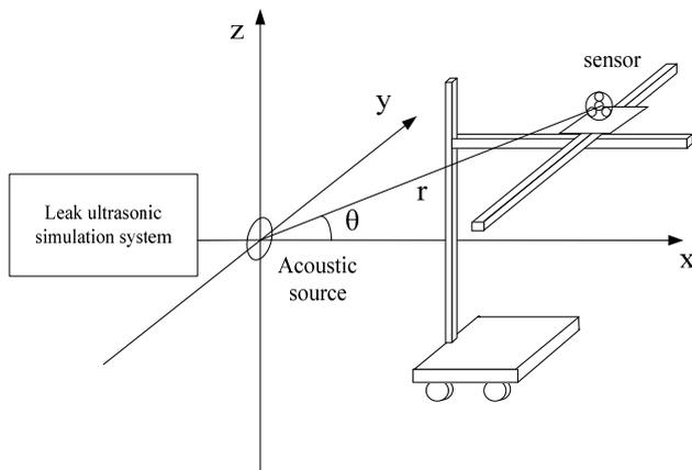
Fig. 3 Diagram of sound pressure test system
