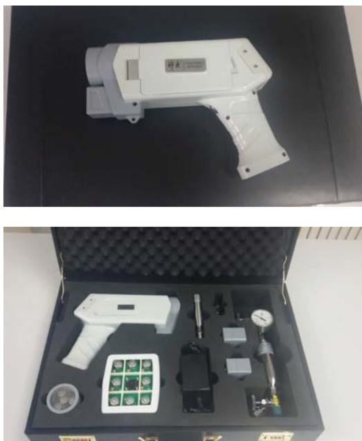
Fig. 9 Picture of the portable ultrasonic leak detector
