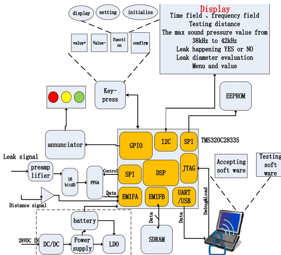
Fig. 8 Diagram of the portable ultrasonic leak detector
