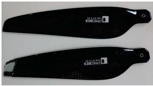
Fig. 8 A propeller with a damaged tip that was used in our experiments
