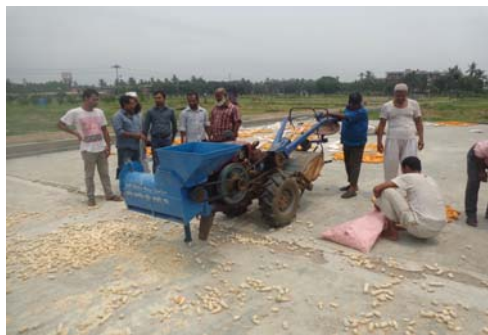
Fig. 5 Operation view of BARI mobile maize sheller
