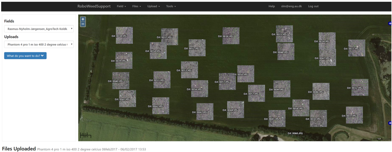
Fig. 3 Images acquired during test of the system performed February 6, 2017 and uploaded to the RoboWeedSupport cloud as described in details by Rydahl et al. [16] The images are plotted corresponding to the location they were taken
