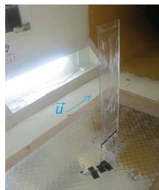
Fig. 2 Experimental setup for PC plate structure in Wind tunnel, Courtesy of Ankara Rüzgar Tüneli (ART)
