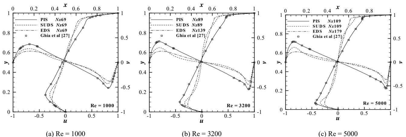
Fig. 5 Velocity profiles in lid-driven cavity flow at mid-sections for various upwind schemes
