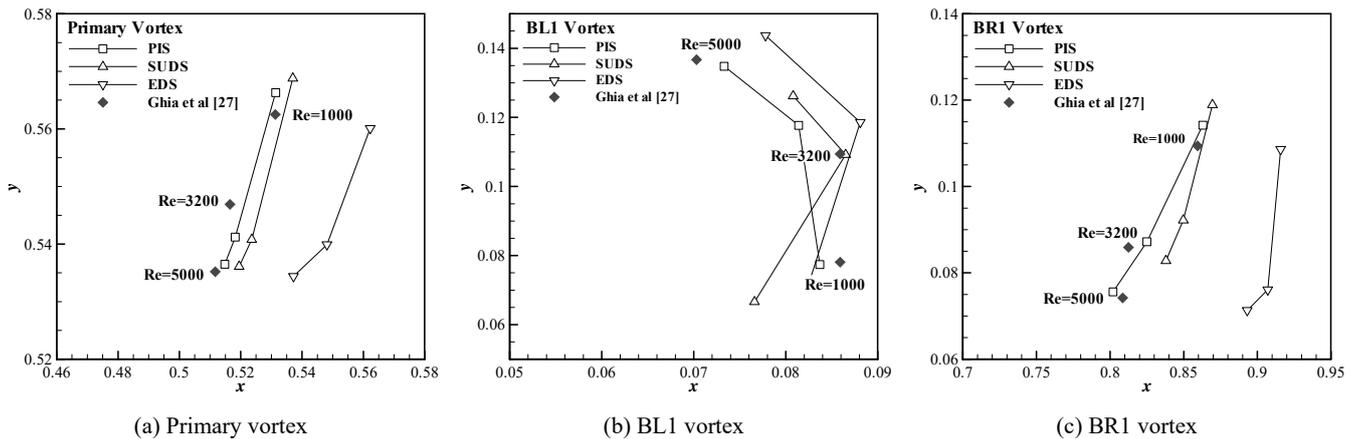
Fig. 7 Coordinates of the center of lid-driven cavity vortices at different Reynolds numbers predicted by the advection schemes
