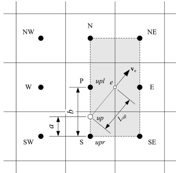
Fig. 2 An element constructed from cell centers surrounding the point  $e$  of cell  $P$ , and representation of the skew upwind point for point  $e$ ; here, cell centers  $S$  and  $P$  are the right (upr) and left (upl) points of the upwind point ( $up$ ), respectively
