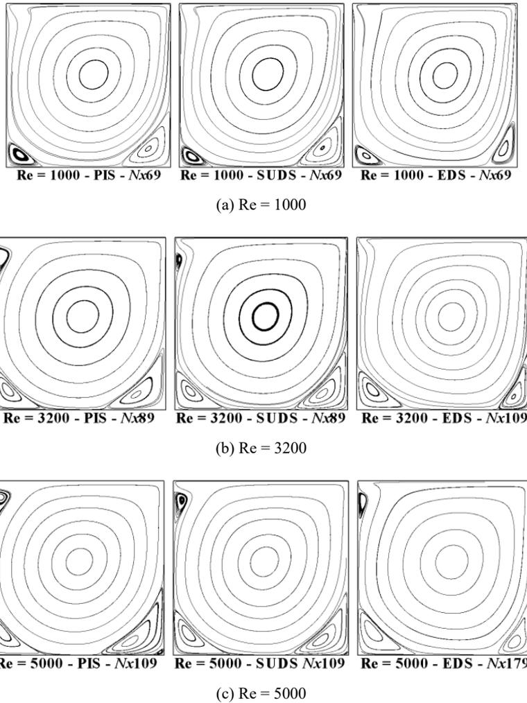
Fig. 6 Streamlines in lid-driven cavity flow for various upwind schemes at different Reynolds numbers.
