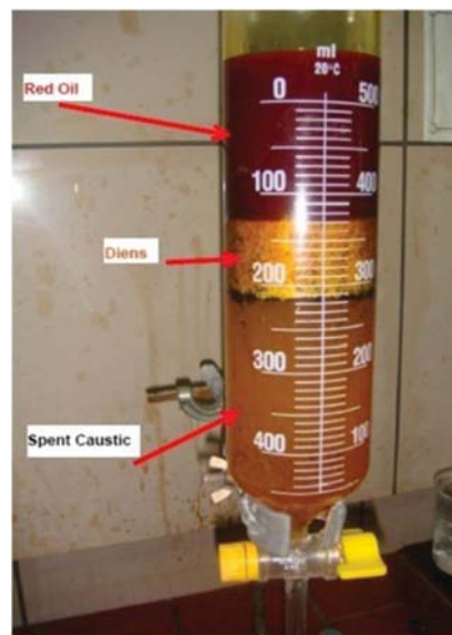
Fig. 1 Separated phases in the tower output sample
