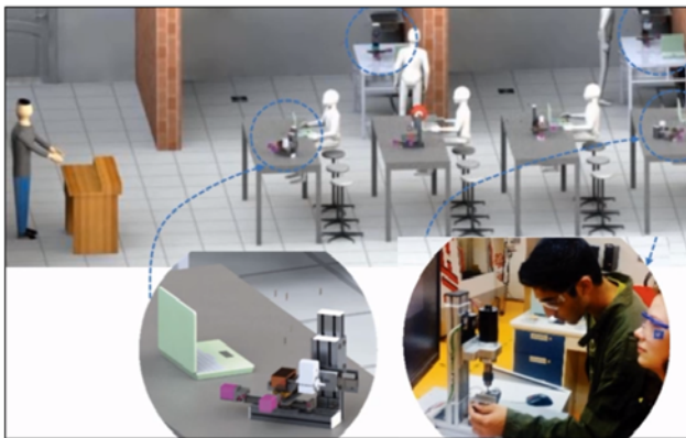
Fig. 6 Prototype of a Reconfigurable CNC Micro Machine-Tool as Cyber-Physical Production System
