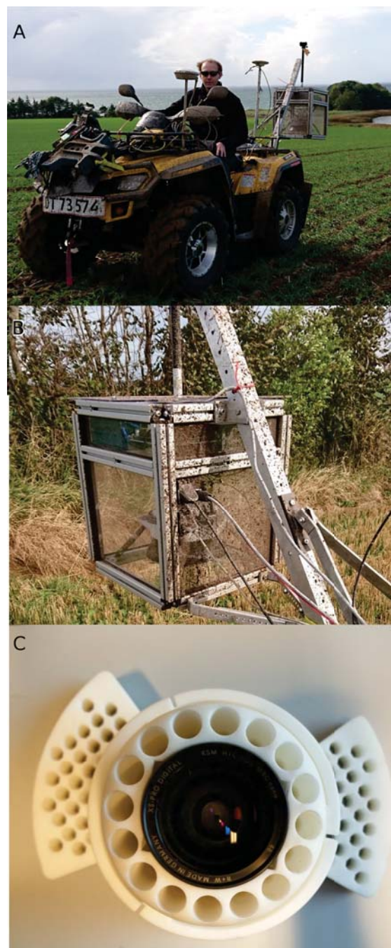
Fig. 1 (A) The ATV mounted up with RTK GNSS and the prototype camera (B) Close up of the high-speed camera after heavy rain during mapping. (C) 3D printed camera bracket
