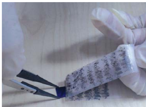
Fig. 4 Scotch tape method of graphene block [20]
