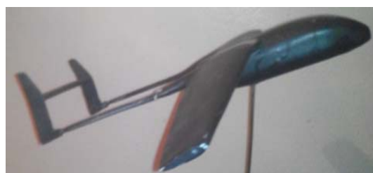
Fig. 2 UAV with an up-horizontal stabilizer and without landing gear
