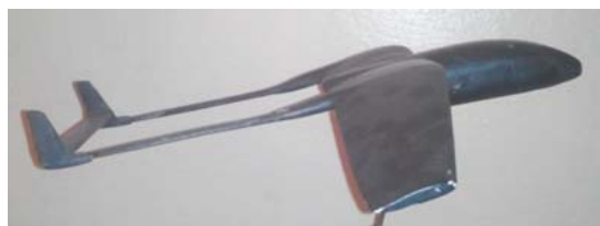
Fig. 3 UAV with a down-horizontal stabilizer and without landing gear
