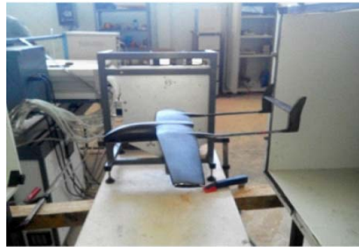
Fig. 5 Model in the wind tunnel
