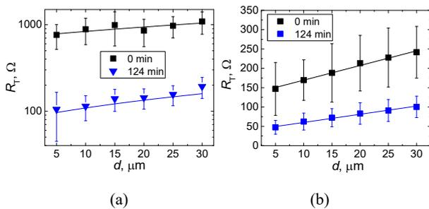
Fig. 3 CTLM resistance versus distance plots for (a) Ni and (b) Au contacts. Total device resistance  $R_T$  dependence on distance between contacts  $d$  before annealing (black curve) and after 124 min annealing (blue curve)
