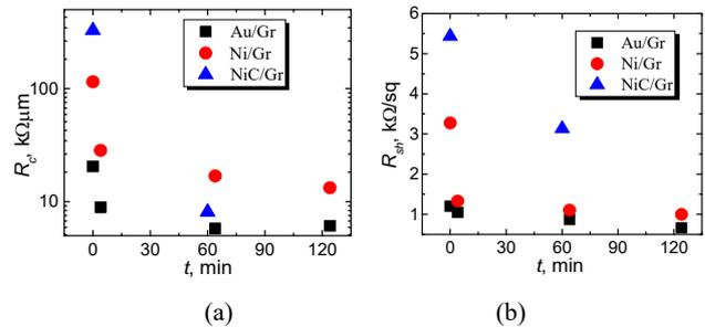
Fig. 4 Average contact resistance  $\langle R_C \rangle$  (a) and average sheet resistance  $\langle R_{Sh} \rangle$  (b) dependencies on rapid thermal annealing time ( $t_{\text{anneal}}$ ) of Au/Graphene and Ni/Graphene contacts: each data point consists of more than 25 experimental values
