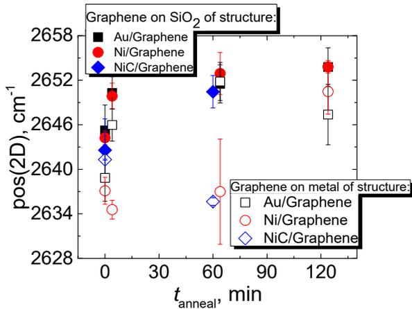
Fig. 8 Raman shift of 2D peak position versus anneal time: solid symbol represents graphene on SiO<sub>2</sub> (between Au (black), Ni (red) and NiC (blue) metal contacts). Unfilled symbol represents Au/Graphene (black), Ni/Graphene (red) and NiC/Graphene (blue) metal contacts
