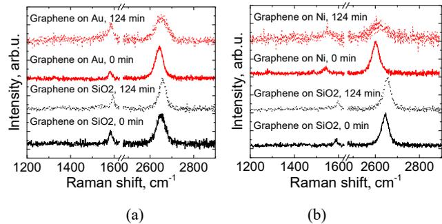
Fig. 7 Raman spectra of graphene transferred on  $\text{SiO}_2$  substrate and metal contacts before annealing (solid line) and after 2h annealing (dots); (a) Raman spectra of graphene transferred on  $\text{SiO}_2$  substrate and Au contacts (b) Raman spectra of graphene transferred on  $\text{SiO}_2$  substrate and Ni contacts
