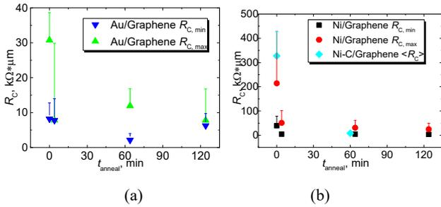
Fig. 5 Variation of  $R_C$  of Metal/Graphene devices versus annealing time (a)  $R_C$  derived from six samples of the lowest and highest resistance of Au/Graphene devices; (b)  $R_C$  derived from six samples of the lowest and highest resistance of Ni/Graphene devices and average resistance of NiC/Graphene devices
