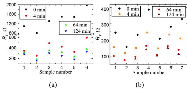
Fig. 2 Comparison of the measured resistances of CTLM structures with 30  $\mu\text{m}$  distance between metal contacts before (0 min) and after 4, 64, and 124 min annealing (a) Ni/Graphene; (b) Au/Graphene
