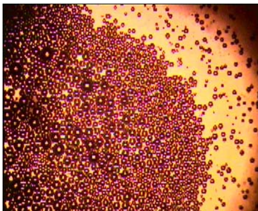
Fig. 10 Optical microscope images with a 100 X magnification of liposomes with a hydrophilic dye after passing through a stacked membrane of pore size of 400 nm
