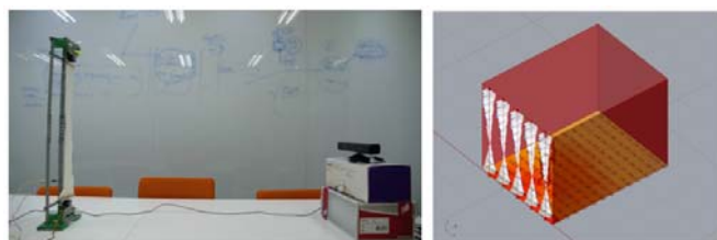
Fig. 4 A Kinect sensor as a 3D scanner digitizing the shape of a physical model [8]
