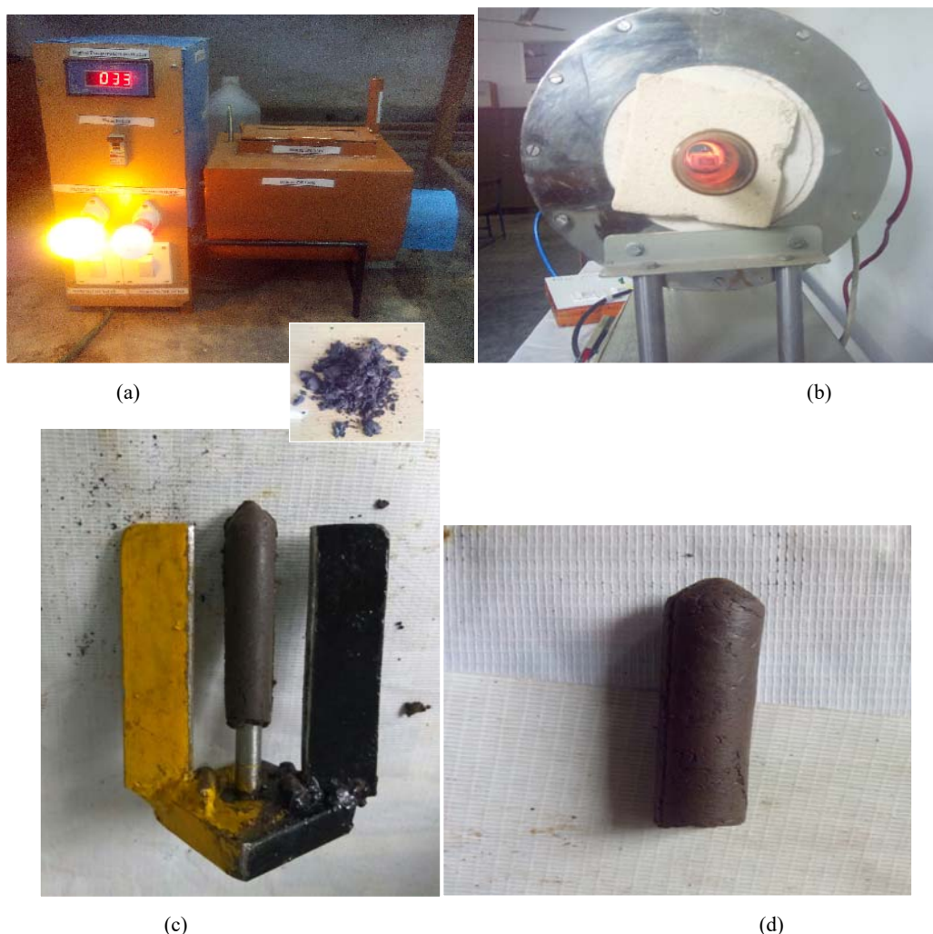
Fig. 4 (A) Fabricated sigma mixer with Green Mixture, (B) Schematic diagram of furnace used for sintering, (C) Green filter sample with dies and (D) Brown filter sample
