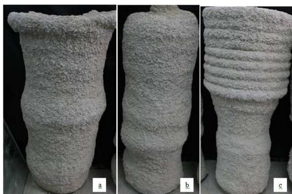
Fig. 4 JG columns produced in (a) 1<sup>st</sup> Combination (b) 2<sup>nd</sup> Combination (c) 3<sup>rd</sup> Combination
