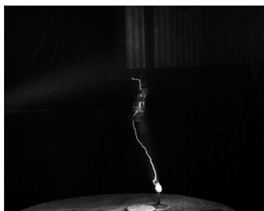
Fig. 5 Characteristic picture of the formation of the main stage of discharge in the gap “positively charged water aerosol cloud – ground” in the presence of the array of the model hydrometeors of cylinder form
