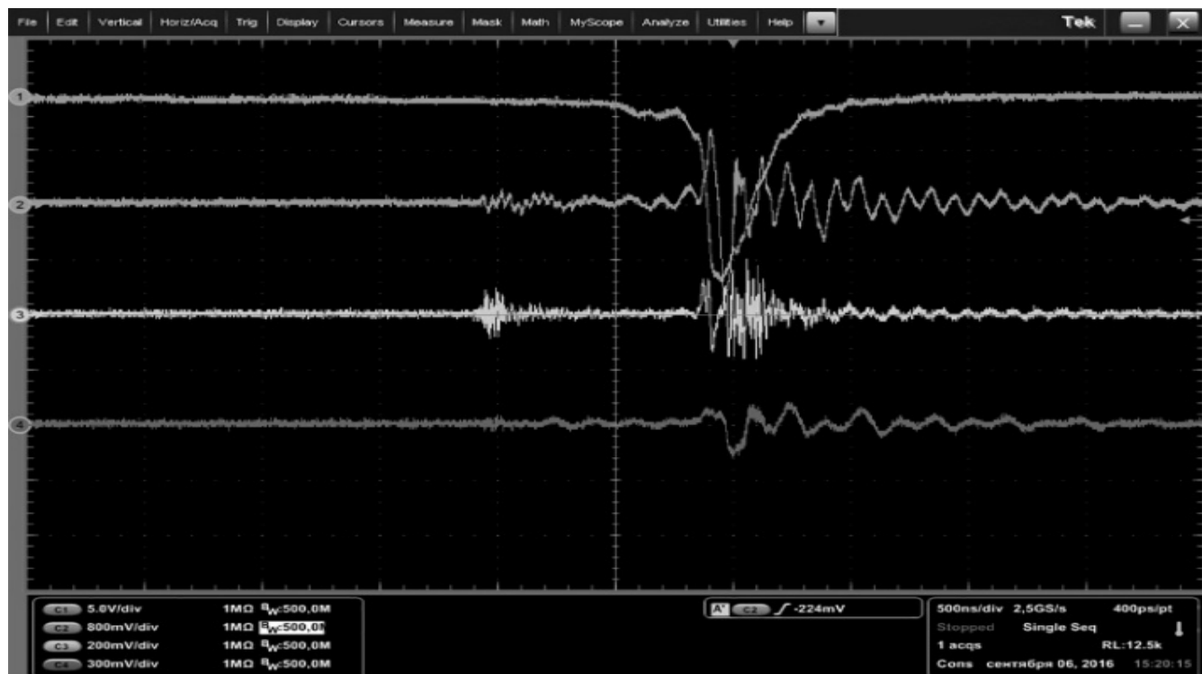
Fig. 4 Oscillograms of the discharge current (curve 1, shunt 0.5 Ohm), of the signal registered by the plate antennas A1 (curve 2, shunt 0.5 Ohm), A2 (curve 3, shunt 0.5 Ohm), A3 (curve 4, shunt 0.5 Ohm) for the main stage of discharge in the gap “negatively charged aerosol cloud – ground” in the presence of the array of the hydrometeors of ellipsoid form
