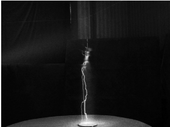
Fig. 2 Channel discharges initiated by the array of cylinder hydrometeors between the positively charged water aerosol cloud and the ground
